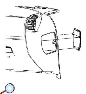
2. Remove the service panel located on the right side of the instrument panel (I/P).
